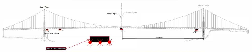
Four 54 ft wide temporary platforms are installed in the main span below low steel of the bridge, in relation to centerline of the span; two south of the north tower and two north of the south tower, reducing vertical clearance by no more than 14 feet. The upstream and downstream lower edges of the temporary platforms will be lighted at night with steady burning red lights visible at 2,000 yards by approaching vessels.
