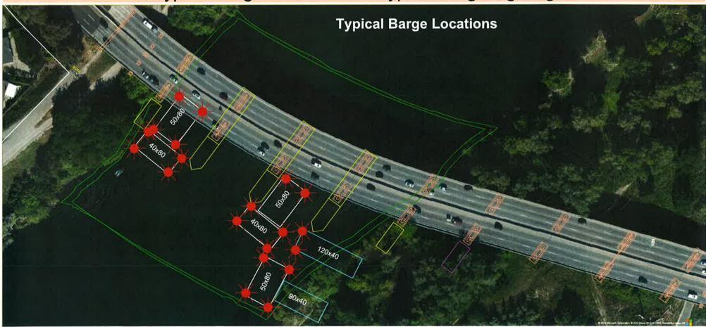
Each corner of each barge is lighted at night with steady burning all-round red light, visible at 2,000 by approaching vessels. All vessels transiting the project area should use extreme caution. Turbidity curtians will be placed at different locations during the project. The next four diagrams show the proposed location of the curtains.
