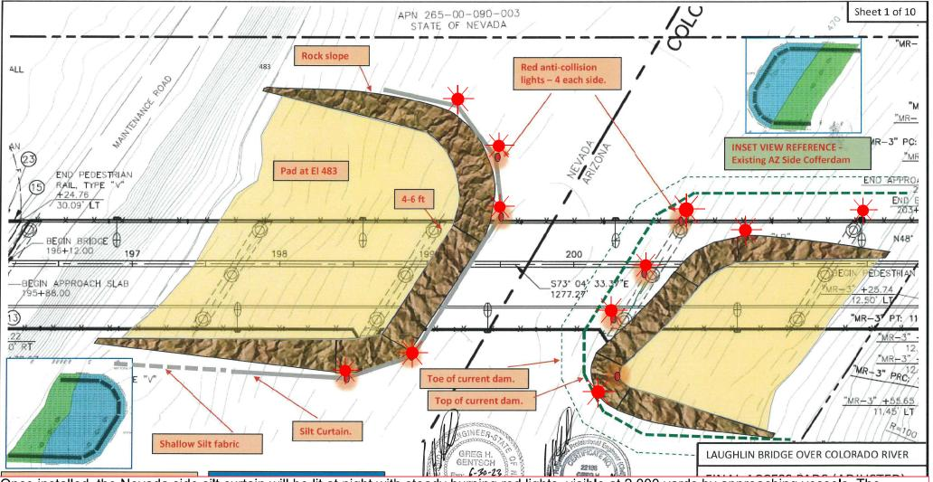
Once installed, the Nevada side silt curtain will be lit at night with steady burning red lights, visible at 2,000 yards by approaching vessels. The Arizona side exposed bridge piers and upstream and downstream ends of the rock access pad will be lit at night with steady burning red lights, visible at 2,000 yards by approaching vessels. There will be approximately 117 feet of horizontal clearance from the face of the silt curtain to the face of the Arizona side pier, in the center of the river.
