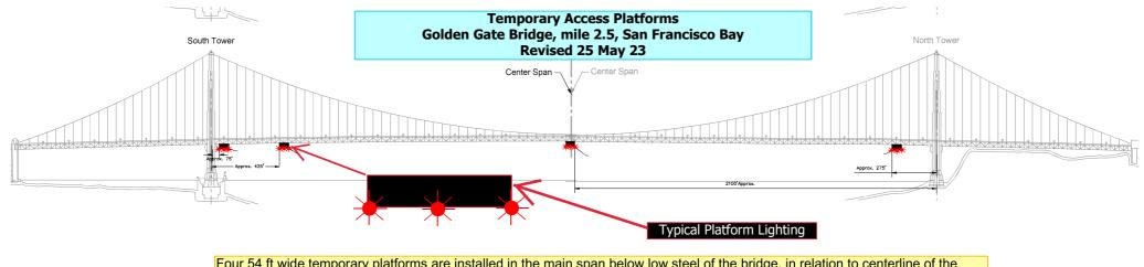
Four 54 ft wide temporary platforms are installed in the main span below low steel of the bridge, in relation to centerline of the span; two south of the north tower and two north of the south tower, reducing vertical clearance by no more than 14 feet. The upstream and downstream lower edges of the temporary platforms will be lighted at night with steady burning red lights visible at 2,000 yards by approaching vessels.
