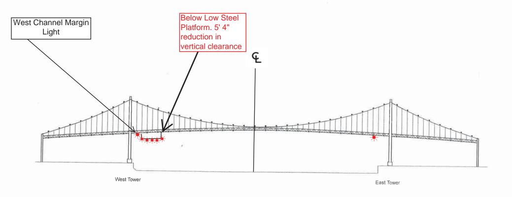
A 180 foot long under deck temporary platform will reduce vertical clearance by 5' 4". Each corner and every 50 feet along the the upstream and downstream side of the platform will lighted at night with steady burning red lights visible at 2000 yards by approaching vessels. In a duration of 1-year the platform will progress from the western channel margin light to 250' west of the centerline of the bridge.
