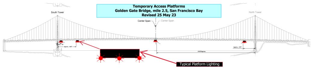
Four 54 ft wide temporary platforms are installed in the main span below low steel of the bridge, in relation to centerline of the span; two south of the north tower and two north of the south tower, reducing vertical clearance by no more than 14 feet. The upstream and downstream lower edges of the temporary platforms will be lighted at night with steady burning red lights visible at 2,000 yards by approaching vessels.
