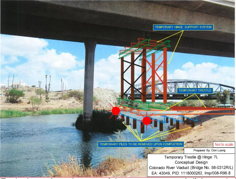
Each channel ward corner of the temporary trestle/falsework is lighted at night with steady burning red lights visible at 1,000 yards by approaching vessels.
