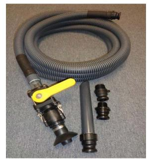
Pumpout wand attachment and supporting parts Photo by KECO Pump & Equipment
