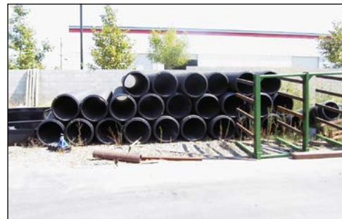
circular pontoons to be foam filled
