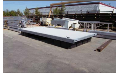
typical 20 ft boarding float section
