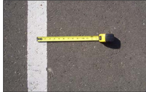
measure to center of painted stripes
