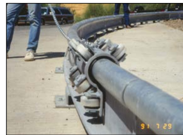
wheeled trolley being tested on a steel pipe rail guidance system --- boarding float not shown
