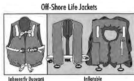
buoyancy. It is effective for all waters, especially open, rough or remote waters where rescue may be delayed. It is designed to turn **most** unconscious wearers in the water to a face-up position.
