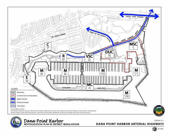
Drive. The posted speed limit is 30 mph north of Dana Point Harbor Drive and 25 mph inside the Harbor entry. Puerto Place, Casitas Place and Island Way are all two-lane undivided roadways trending in a north-south direction; on-street parking is prohibited and a posted maximum speed of 25 mph.
